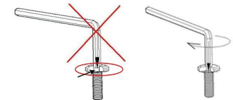
If you don't do that and slip out of the screw, the screw will suffer damage and it can cause the screw head to become round inside so that you won't be able to find grip with the hex key anymore. Round spun screw heads only result from this and aren't a reason for complaints.
