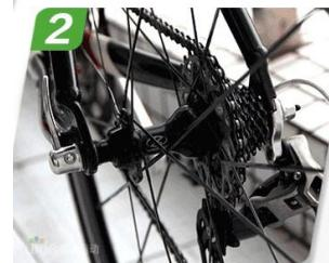
Step 2: Replace the rear axle's quick release lever with professional bike trainer's quick release lever.
