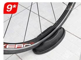
Step 9: The front wheel pad is used to prevent the bicycle from swinging. The pad is random.
