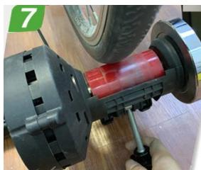
Step 7: Adjust the pressure regulator till it touches the tire. The tightness of pressure regulator determines the resistance force. The tighter, the greater the force is.
