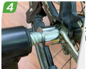
Step 4: Hold the left side of rear axle in connection with the bike trainer's left bayonet.
